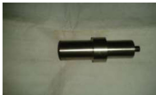
Figure 2.Straight cylindrical FSW tool
