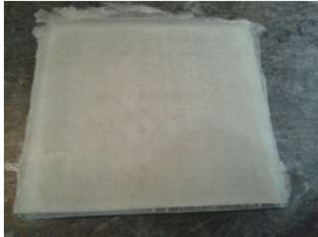
Fig.2.3 Prepared Honeycomb Sandwich (Honeycomb Core between 2 Face sheets
