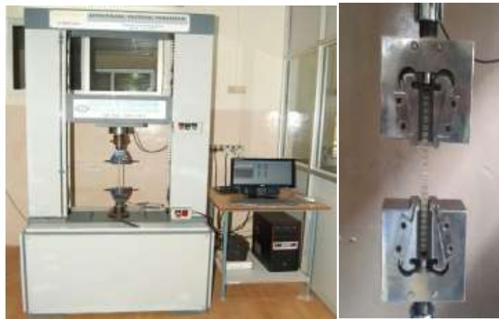
Fig.3.1 Universal Testing Machine (UTM) Setup & Tensile Test Specimen during the Test
