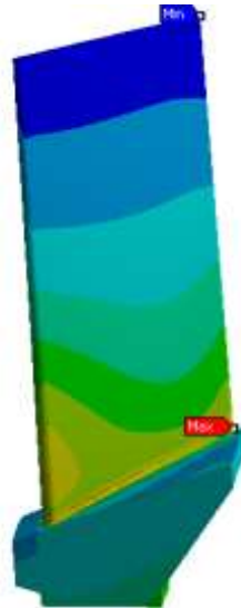
Figure 6: a single sector model showing the equivalent stresses
