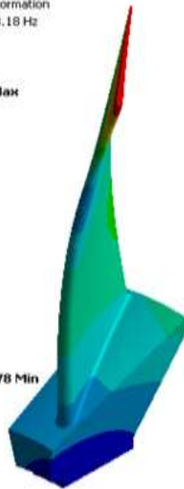
(c) 3 rd mode shape (First flip)
