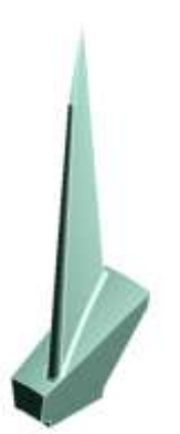
Figure 3: The computer-aided model (CAD) of a single sector turbofan
