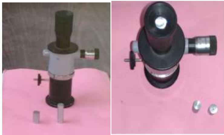
Fig 2: Micrometer microscope with both the specimens
