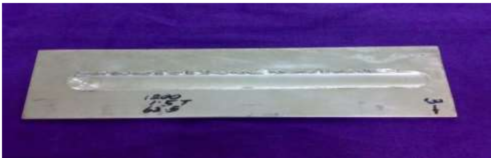
Figure 5.1.3 S1200 Experiment Bead-On Welded Plate
