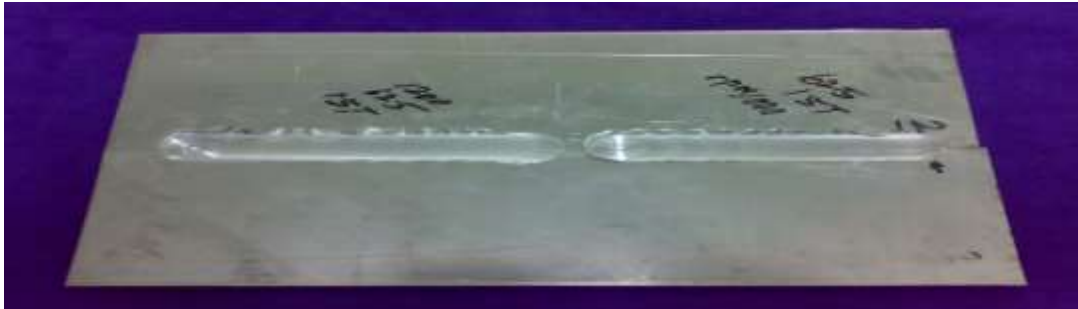
Figure 5.1.2 S1000 and S1200 Experiment Butt Welded Plates
