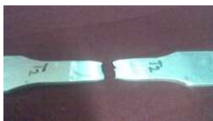
Figure 5.3.1 Tensile Tested Weld Specimen
