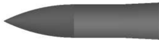
Fig.2 3-D view of Fuselage without spike
