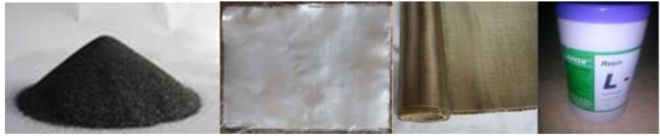
Figure 1: Silicon carbide, Glass fiber, Basalt fiber, and Epoxy
