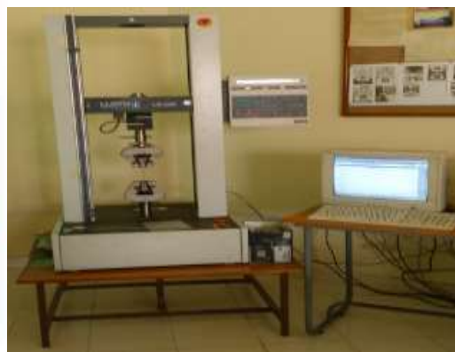
Figure 3. Tensile testing setup
