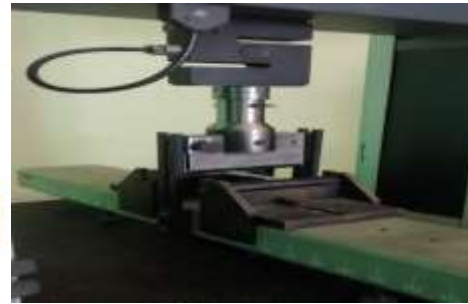
Figure 5. Flexural testing setup
