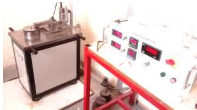
Figure 7. Wear testing setup
