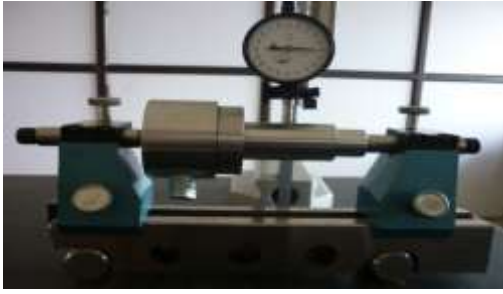
Fig 7.1 Checking the accuracy using Dial Gauge
