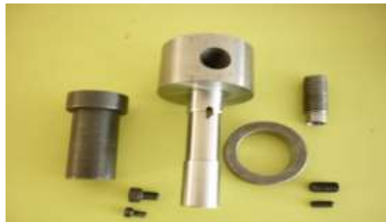
Fig 3.9. Parts of the Hydraulic Expanding Mandrel
