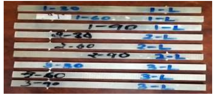
Figure 4: Compression test specimen for different layers of glass fibres.
