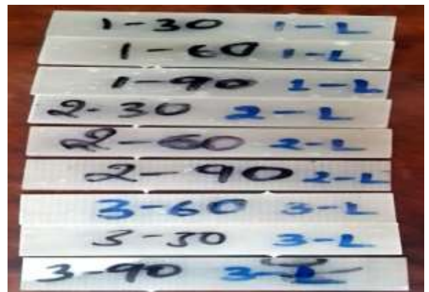
Figure 6: Bending test specimen for different layers of glass fibres.
