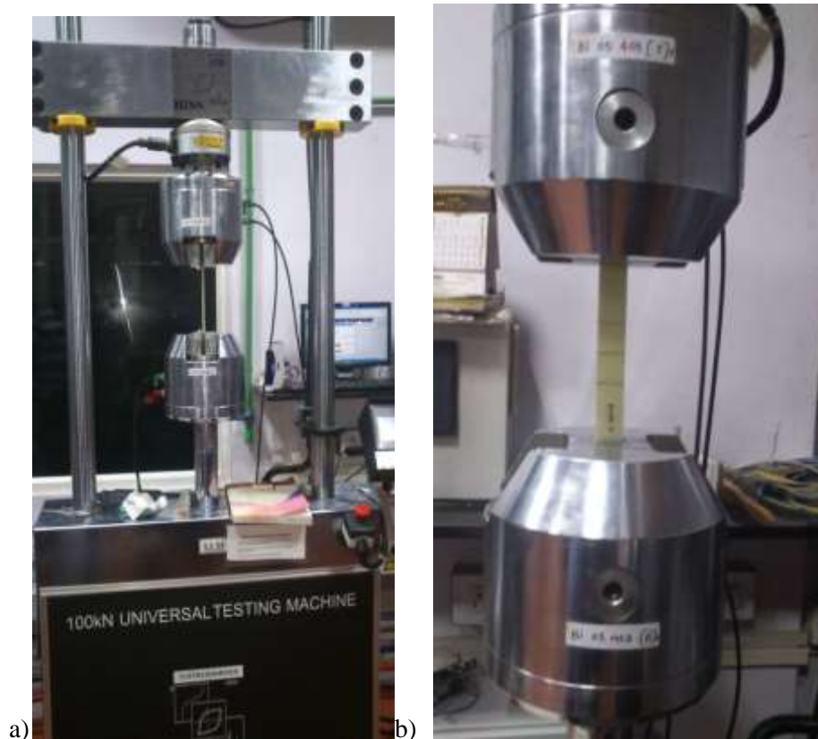
Figure 3. a) Fatigue machine b) Specimen arranged in Fatigue machine.
