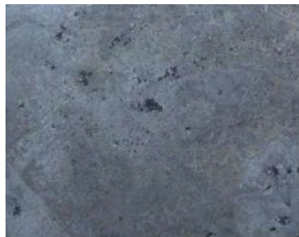
Figure 3: Corrosion pits on the flat surface of as-cast specimen tested for 1 month.
