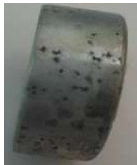
Figure 2: Initiation of corrosion pits on the lateral Surface of as-cast specimen tested for 1 month
