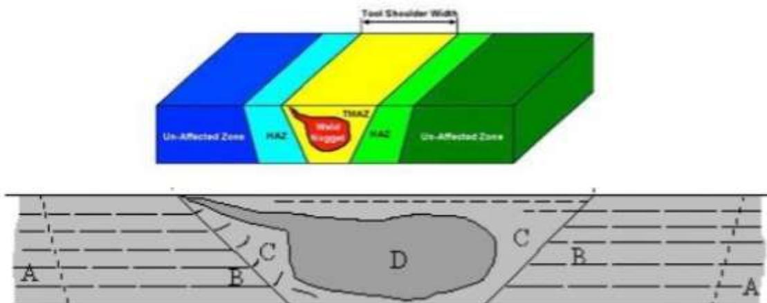
Figure1.2: Microstructure classification of FSW
