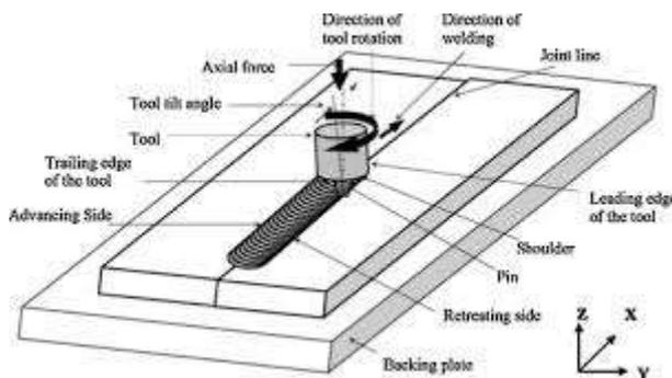
Figure 1.1: Friction Stir Welding Process
