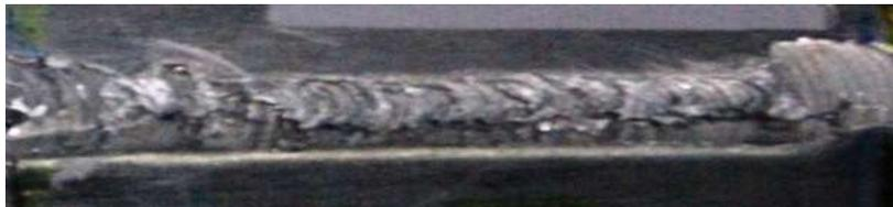
**Figure 3.6: Surface View of the Weld Specimen**
