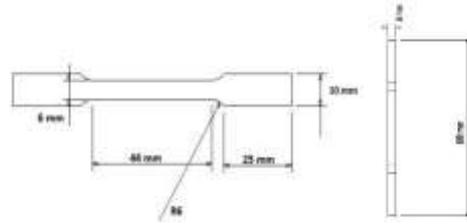
Figure 4.1: Standard Tensile Specimen Dimensioning and Tolerance as per ASTM E8/E 8M-08
