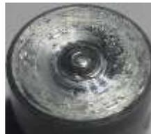
**Figure 3.4:Worn Out Tool Pin**
