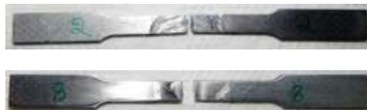
Figure 5.1: Tensile Tested Fracture Specimens
