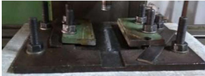
Figure 3.1: Fixture to hold the Workpieces
