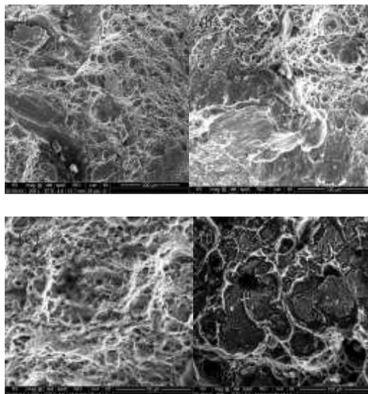
**Figure 7.1: SEM-EBSD Characterised Micrographs of Fractured Tensile Specimens: (a) Intermetallic Compounds surrounding Equiaxed Grains in Stir zone; (b-d) Equiaxed Dimples away from Nugget;**
