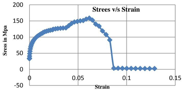
**Figure 5.3: Stress-Strain Behaviour of Trail No.8 Tensile Specimen**
