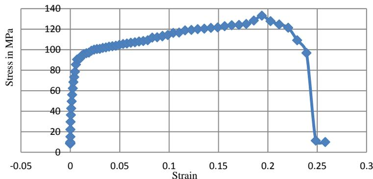
Figure 5.2: Stress-Strain Behaviour of Trail No.2 Tensile Specimen
