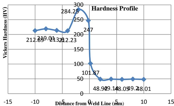
**Figure 8.1: Vickers Microhardness Distribution Profile along the Weld Cross section Trail No.2**
