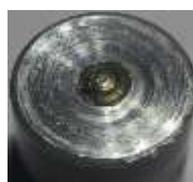
Figure 3.10: Worn Out Tool Pin
