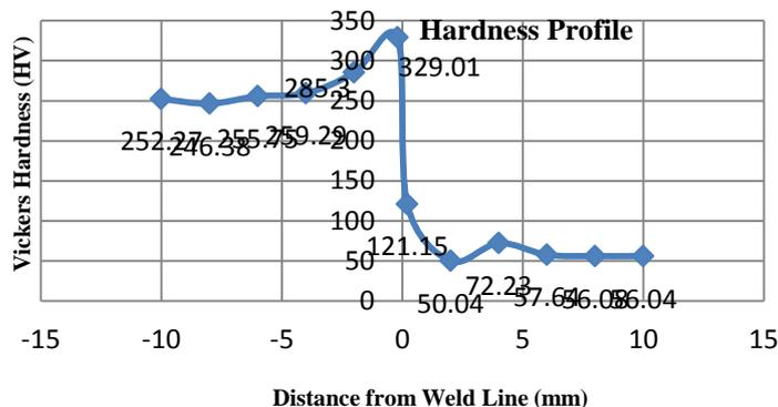
Figure 8.2: Vickers Microhardness Distribution Profile along the Weld Cross section Trail No.8
