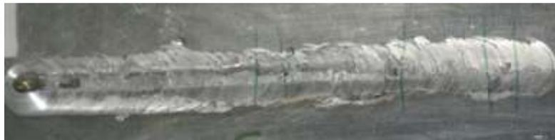
Figure 3.8: Surface View of the Weld Specimen
