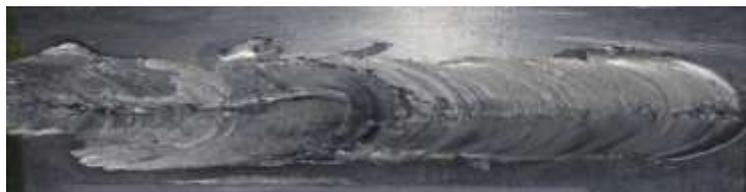
Figure 3.9: Surface View of the Weld Specimen
