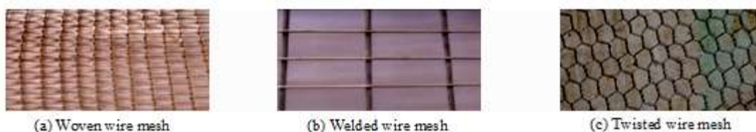
Fig. 4 (a), (b) & (c) Mesh reinforcement espoused for mortars
