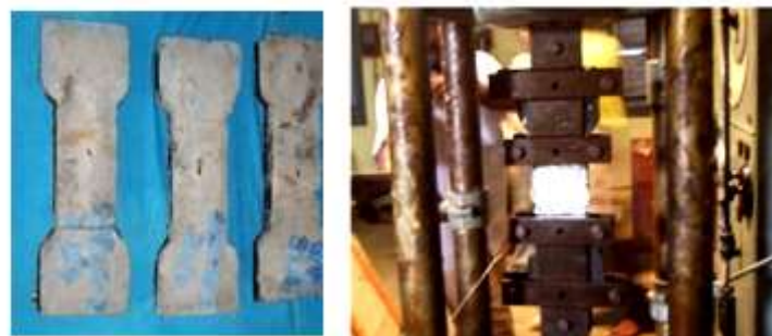
Fig. 7 Tensile specimens along with tension test setup
