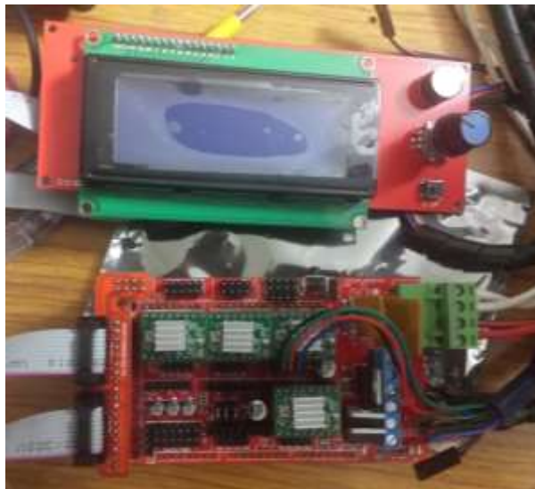
Figure II: electronic assembly used to control the 3D printer
