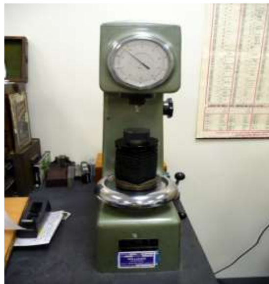
Fig 3.1: Rockwell Hardness Setup
