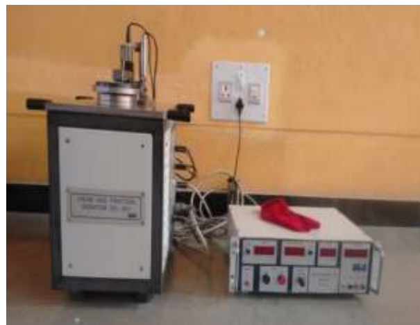
Fig 3.2: Pin on Disc Setup
