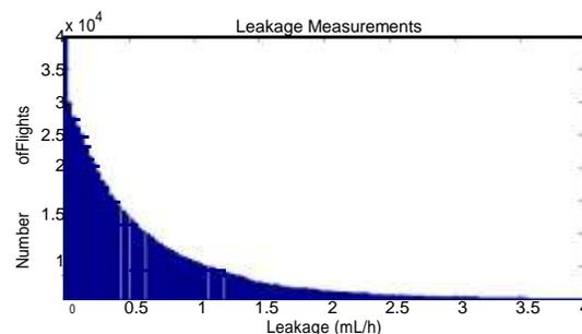
Figure 7 Fleet leakage estimation histogram.
