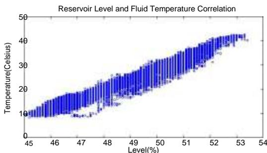
Figure 4 Relation between temperature and reservoir level.
