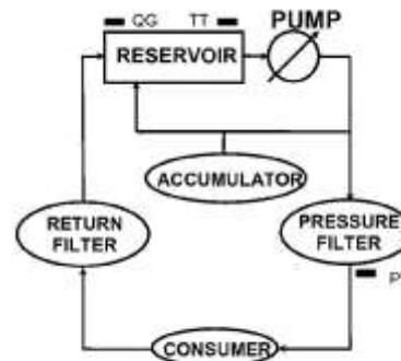
Figure 1 General Schematic of a Hydraulic System
