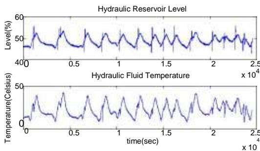
Figure 2 Hydraulic system flight record example.
