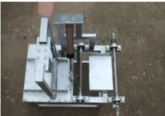
Fig 7 : Working Model of sheet metal cutting & bending machine
