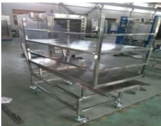
Fig.12 Multi Level loading trolley for loading parts
