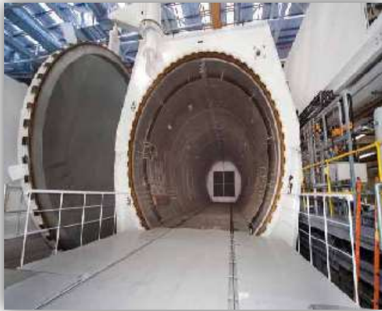
Fig.2. A typical Autoclave used to cure composite parts.
