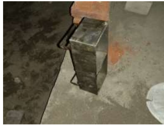
Figure No..7 Mould: Steel Box
