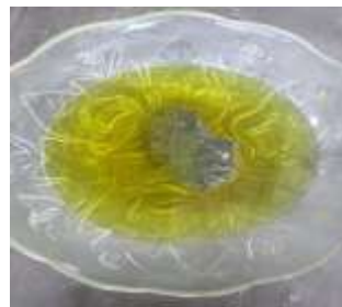
Figure No..14 Brick In Acid (Glass Vessel)
