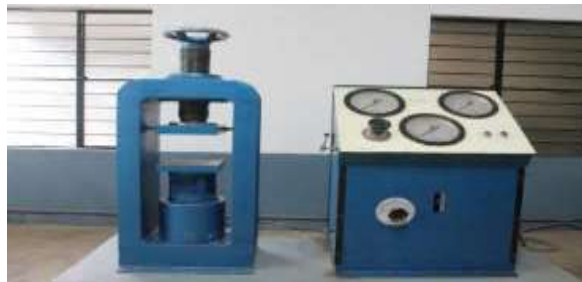
Figure No..10 Hydraulic Brick Testing Machine
