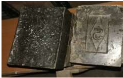
Figure No..1. Brick 70% Sand(River Gravel Sand) + 30% Plastic Waste
