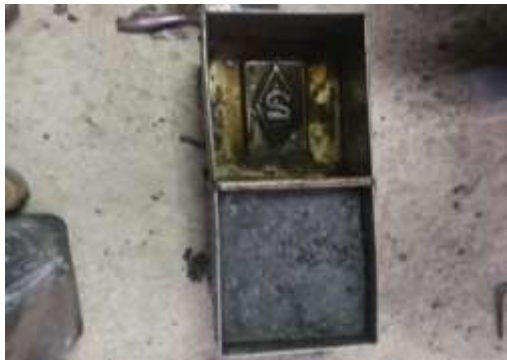
Figure No..8 Brick In Mould Kept For Cooling
