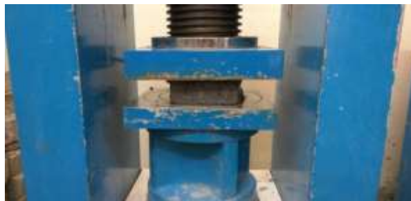
Figure No..11 Brick Testing
