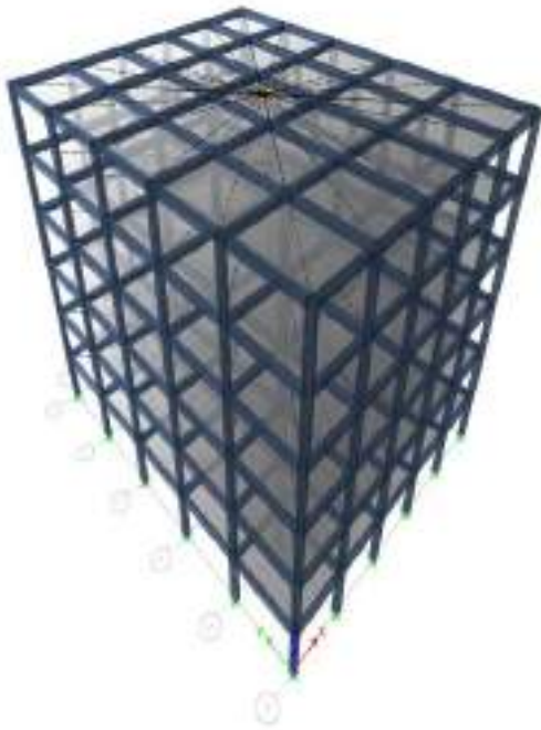
Figure 2.3: 3D view of 6-story regular RC building
