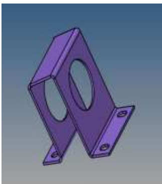
Fig.9 LH bracket with increased thickness
