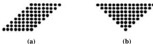
Fig 2 Dotted representation of partial products for 8-bit multiplier
