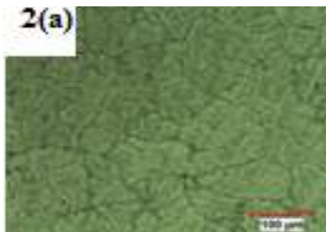
“Fig. 2(a),” Optical microscope images of Al 2219 alloy
