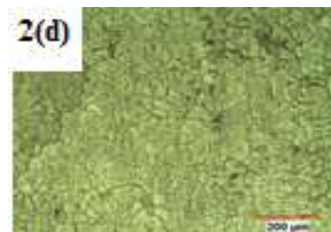
“Fig. 2(d),” Optical microscope images of Al 2219+5% Al 2 O 3 +5% MoS 2 .
