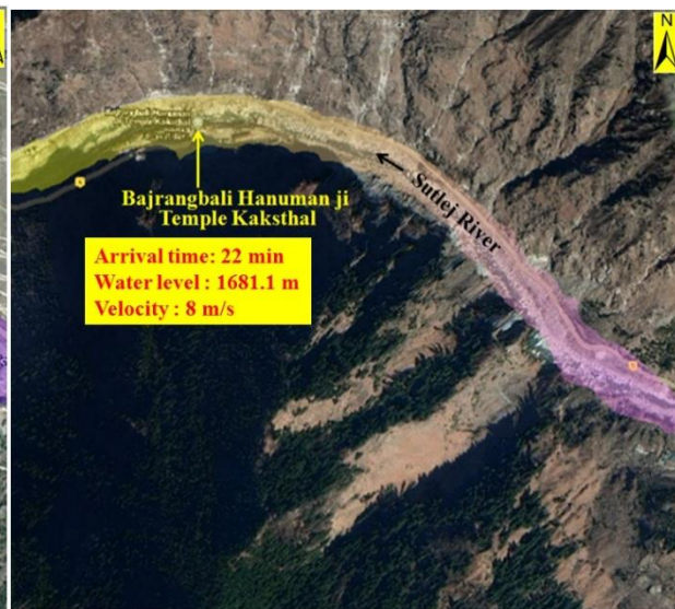
Figure.7: Bajrangabali mandir-16.73 km d/s of dam
