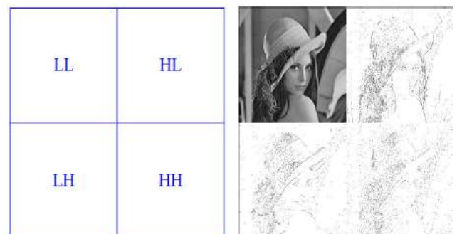
Figure.7 DWT of image from [5]
