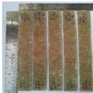
**Fig. 5:** Specimens for before the tensile test (ASTM 3039)
