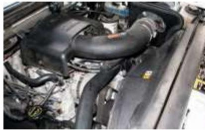
Figure 2. Hoses fitted in an I.C. engine
