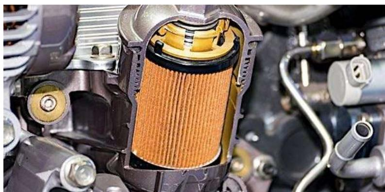
Figure 3: Oil Filter [Type: Cartridge]
